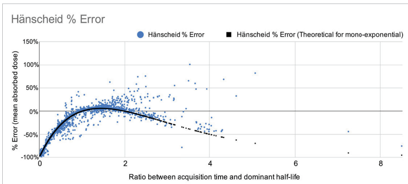
FIGURE 4. Single-timepoint dose error as a function of t_{\text{acq}}/T_{\text{eff}} . Results across all ROIs, cycles, and patients from this evaluation are plotted in blue. The theoretical curve for a mono-exponential decay assumption is plotted in black.
